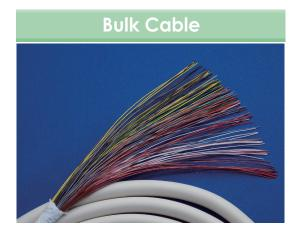
A wide range of probe cables are available, ranging from low capacitance types up to 42AWG and high capacitance types up to 44AWG. They are not only fine, but are also designed to keep excellent transmission performance with lower loss using high conductivity copper-alloy conductors and thinner foamed insulation with low-dielectric constant.
